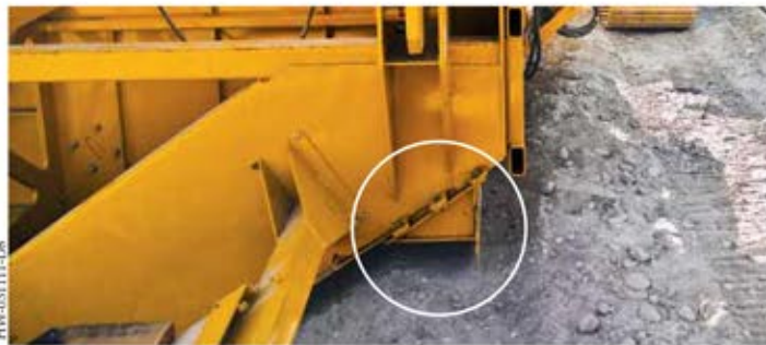
An adjustable berm cap is available on the canal mold. The adjustable berm cap is attached to the pan and can be adjusted by sliding the mechanism up or down and then bolting it into place.
