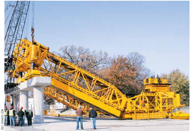
GOMACO's testing pier in Ida Grove, Iowa, U.S.A., simulates the slope of the canal and allowed engineers to test the different operations of the canal equipment and their many specially-designed features.
