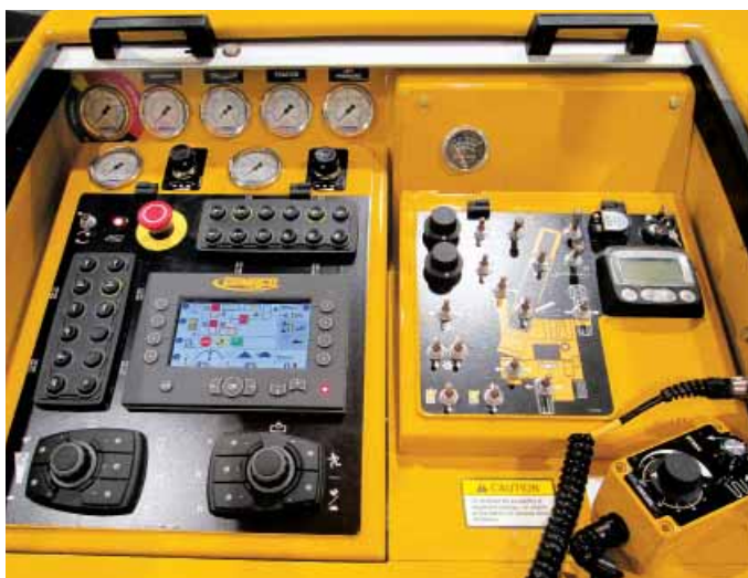
GT-3600 curb and gutter slipform paver with the G+ control system.
