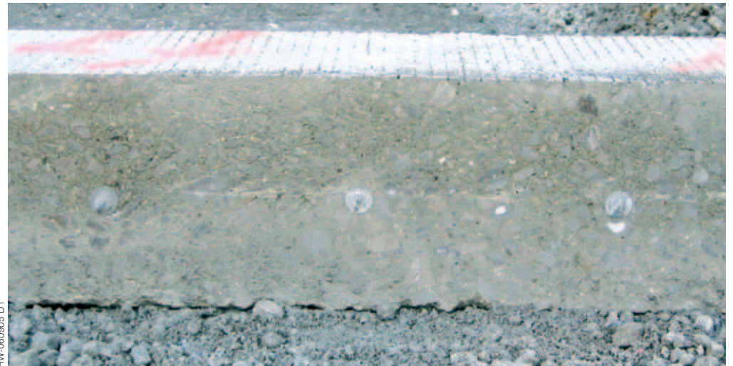
Test headers with the IDBI system inserting a transverse joint were saw cut through the joint and horizontal and vertical tolerances were measured for bar placement. John Carlo had no problems achieving bar placement accuracy.
