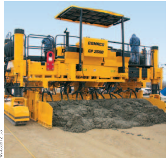
The Turkish Air Force conducts some test pours with their new two-track GP-2600 slipform paver prior to start up on their project in Turkey.
