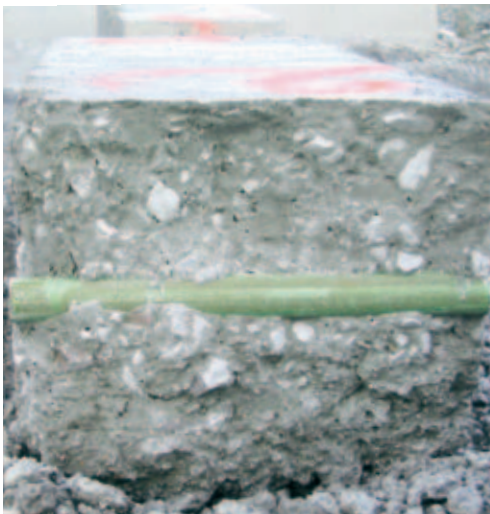
A DOT test shows the bar in the proper horizontal placement with concrete compaction all around the bar.
