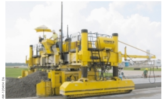
The GHP-2800 paver is slipforming 18.75 feet (5.7 m) wide and 15 inches (381 mm) thick.
