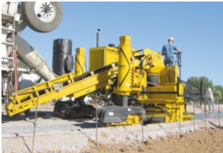
Muse pretrimmed the project 5.5 feet (1.7 m) wide and within a .25 inch (6 mm) tolerance with the GT-3600.
