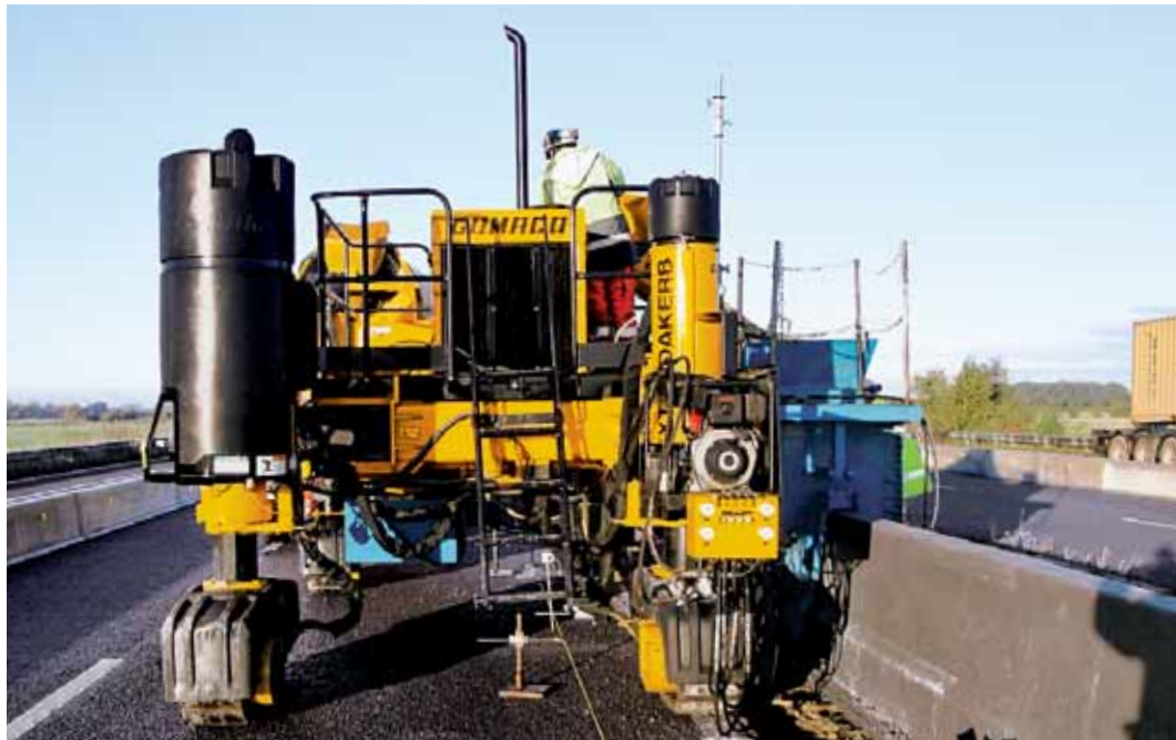
The hydraulic system design of the 4400, along with the effectiveness of load-sensed pumps, proportional solenoids, and the G+® control system, helps to optimize fuel efficiency for a minimum of 18 hours of operation per tank.
