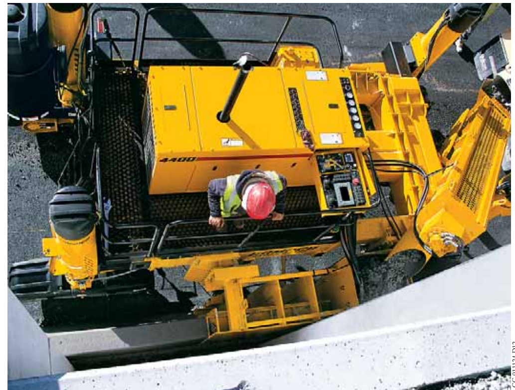
The 4400's U-shaped operator's platform, with vibration isolation, puts the operator comfortably on top of the action. The U-shaped platform and side-to-side sliding console accommodate right-side and left-side pour and provide a 360 degree view of the entire paving operation.
