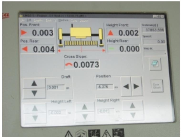
The Leica MPC4 computer is mounted on the GOMACO machine and supplies the operator with system information.
