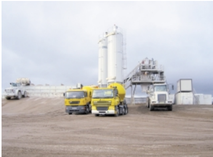
A batch plant sold by GOMACO International Ltd. produces up to 157 cubic yards (120 m 3 ) per hour of concrete.
