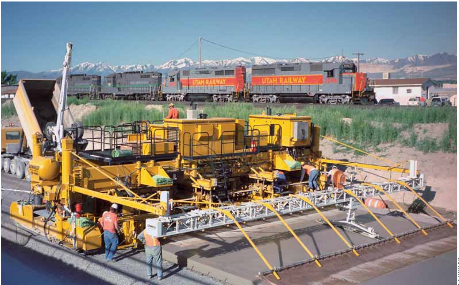
The two-track GP-4000 is equipped with the world's most accurate IDBI system. GOMACO's patented IDBI dowel bar inserter provides ease and accuracy in dowel bar placement transversely across the slab. This machine is also equipped with a sidemounted air-powered bar inserter and will accommodate most types of bars. Optional 16 foot (4.88 m) or 18 foot (5.49 m) track lengths are available for customer preference.
