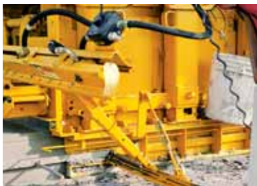
Male keyway with side bar inserter (SBI).
