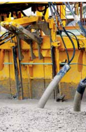
GOMACO's sideplate extension with the hydraulic system bar inserter.
