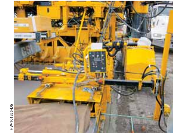
The 5400 series bar inserter is front or rear loading and front inserting for ease of use. It mounts to the mold's T-bar and allows on-the-go crown changes, while maintaining a constant depth. The bar box is mounted to the paver's rear T-beam mounting rail for easy access and loading of the bar magazine. There are individual depth guides on the right and the left side of the bar inserter in order to keep bars parallel to the top of slab. The 5400 series bar inserter can hold up to 50 bars in the bar magazine and bar loading chain system.
