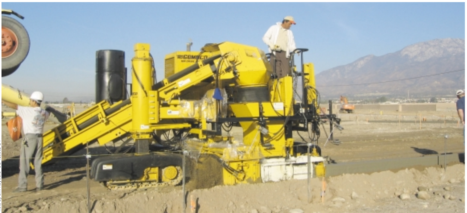
A mold from the company's Commander II was modified to fit the GT-3600. Timing constraints didn't allow for a new mold.
