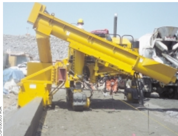
A new generation Commander III with a rear-mounted auger finishes a test pour in Toulnoustouc, Quebec, Canada. Aecon will be slipforming inverted stairway to form the sides of a dam.
