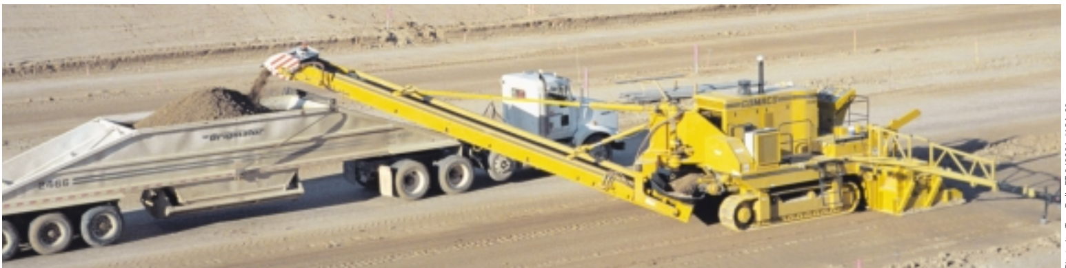
GOMACO trimmers can either discharge into haul units for easy removal or over the stringline for backfill material.
