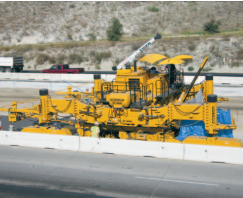
The right front track and two rear tracks on the GP-4000 paver had six foot (1.8 m) leg extensions.
