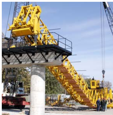
The paver and work bridge for the All-American Canal sits on the pier at GOMACO's testing facilities in Ida Grove, Iowa.
