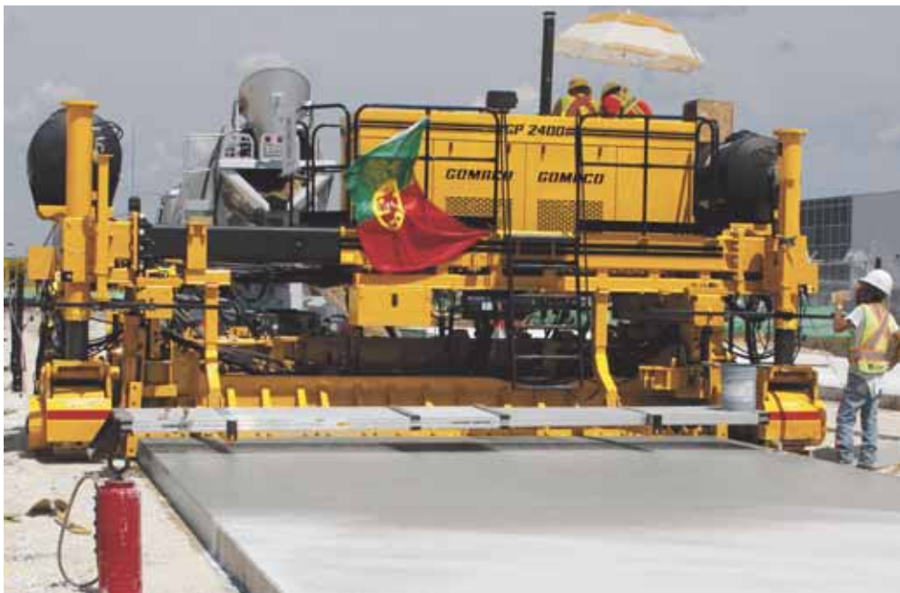
Bituminex Paving Ltd. slipforms 16 feet (5 m) wide with their new GP-2400 paver on a parking lot project in Winnipeg, Manitoba, Canada.
