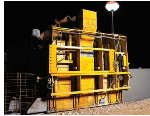
The GOMACO barrier mold features a hopper that telescopes for hydraulic height adjustment.
