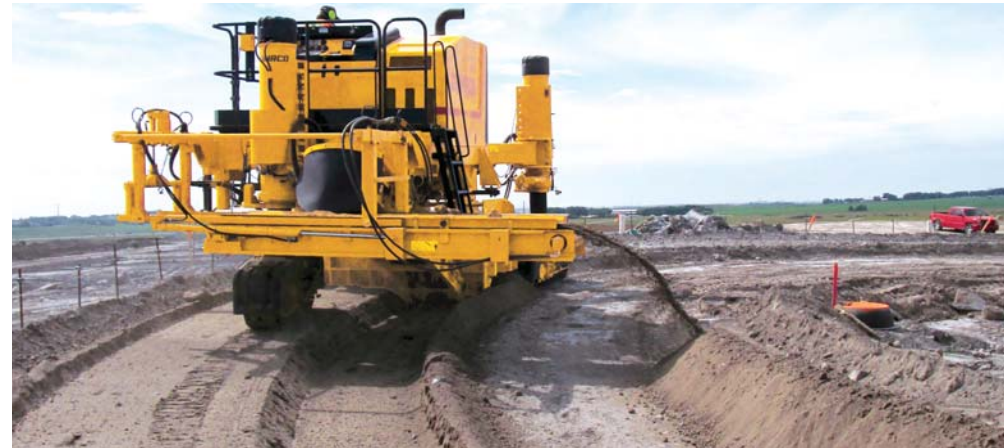
The Commander III sidewalk trimmer features an undermounted trimmerhead capable of preparing grade for flat or monolithic sidewalk up to 11 feet (3.4 m) wide.
