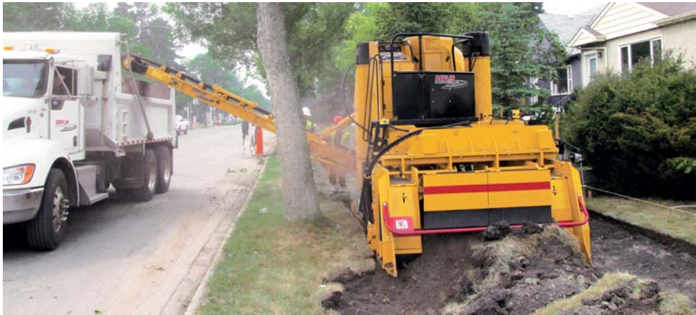
The GT-3400 sidewalk trimmer is operated with a wireless remote control, features a folding and swinging conveyor, and a hydraulically-controlled front gate to trim through windrowed material.
