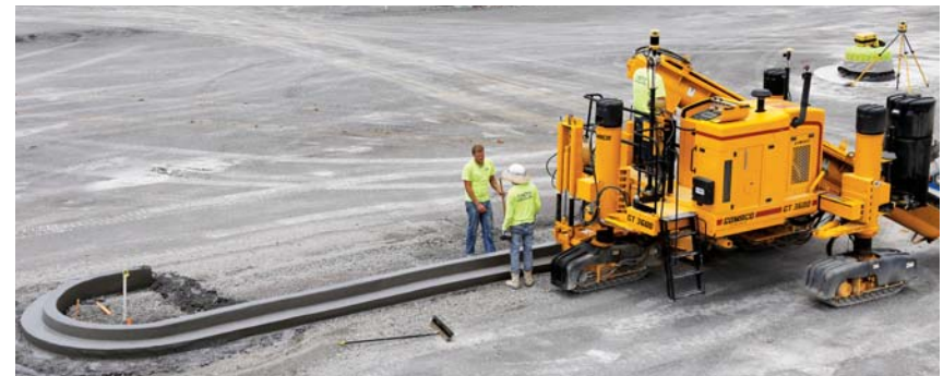
The GT-360's All-Track Steering, combined with Topcon's steering algorithms, allow for smooth entrances and exits and tighter cornering for tight radii work on parking lots.
