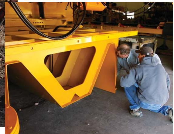
The water channel's large profile was designed to withstand ground movement caused by dynamite blasting from a nearby surface coal mine complex.
