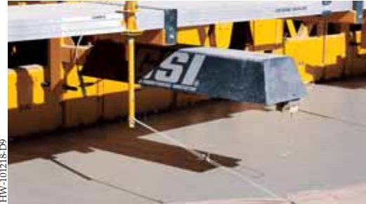
A paver-mounted GSI unit provides immediate monitoring to assure proper paver set up and performance or examine for corrective measure that need to be taken.
