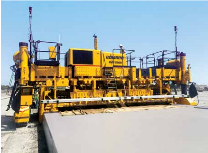
The GOMACO four-track GHP-2800 is equipped with Topcon 3D stringless guidance to pave an airport project 25 feet wide (7.62 m) and 22 inches (56 mm) deep.
