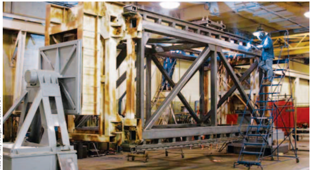
GOMACO workers assemble and weld the 10 foot (3 m) tall canal paver framework.
