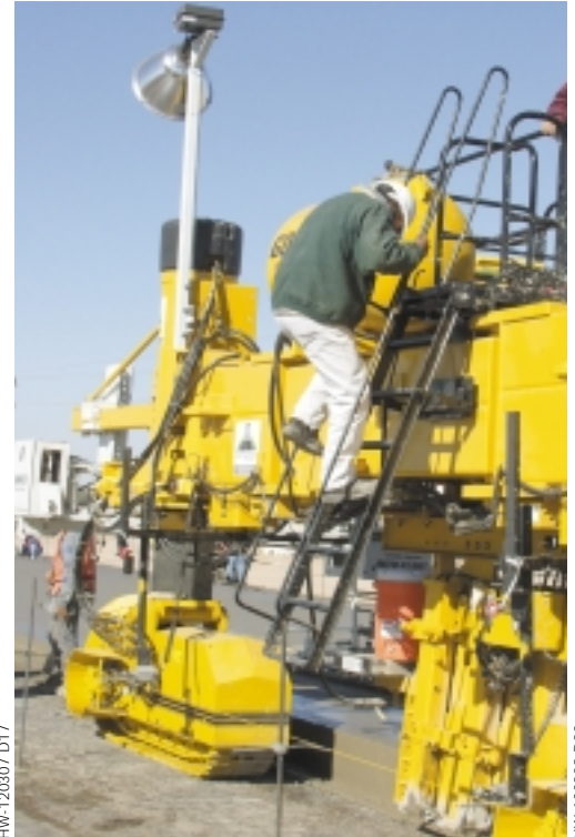
The three-position pivoting ladder can be positioned tight against the paver or tilted out for easier climbing to the platform.
