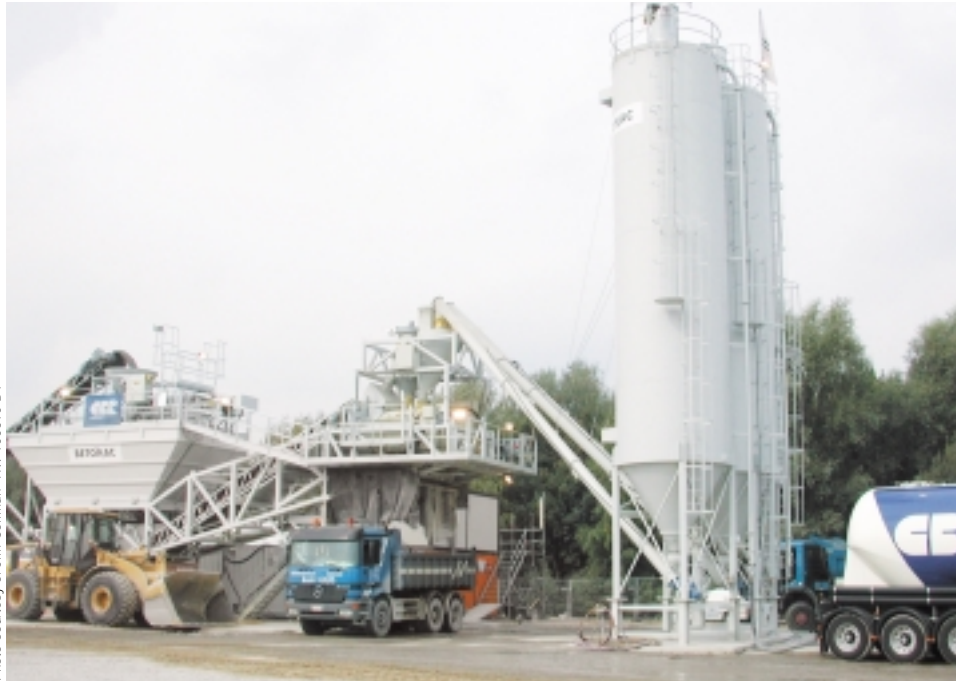
Two Compactor batch plants were on-site providing concrete for the project. Since paving was carried out 24/7, each plant operated in 12 hour shifts. GOMACO International Ltd. is an agent for Compactor batch plants in the UK.
