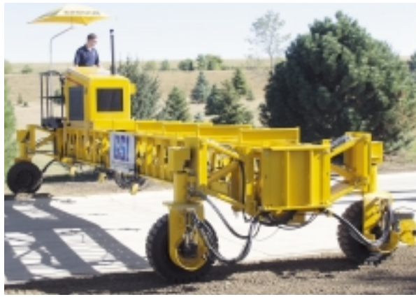
GOMACO's GSI is designed for anyone who needs to measure the smoothness of a surface.
