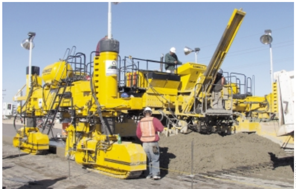
The new generation GHP-2800 four-track is equipped with smart steering cylinders that aid in paver setup and operation.
