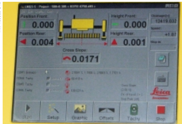
A Leica computer is mounted next to the G21 controller. Information from the sensors and paver logistics are displayed on the monitor.
