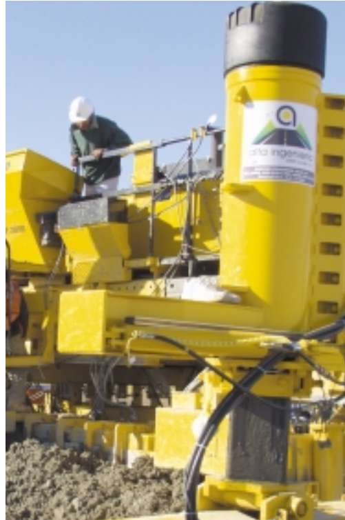
The new generation GHP-2800 four-track is equipped with smart steering cylinders that aid in paver setup and operation.
