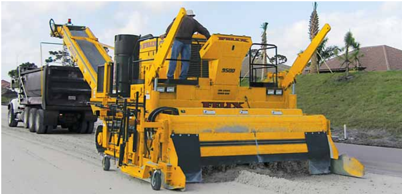
Rolling grade skis are equipped with a sensor wand and traces the existing grade or surface.
