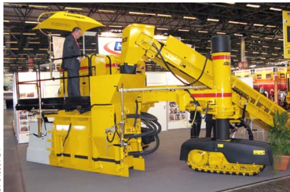
The GT-3200 with right-side mounted barrier wall. It was also on display at Intermat 2009.
