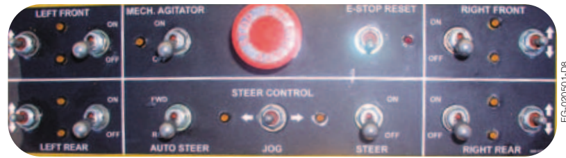
Control box is strategically positioned to provide easy steering control and safety with the emergency stop switch.
