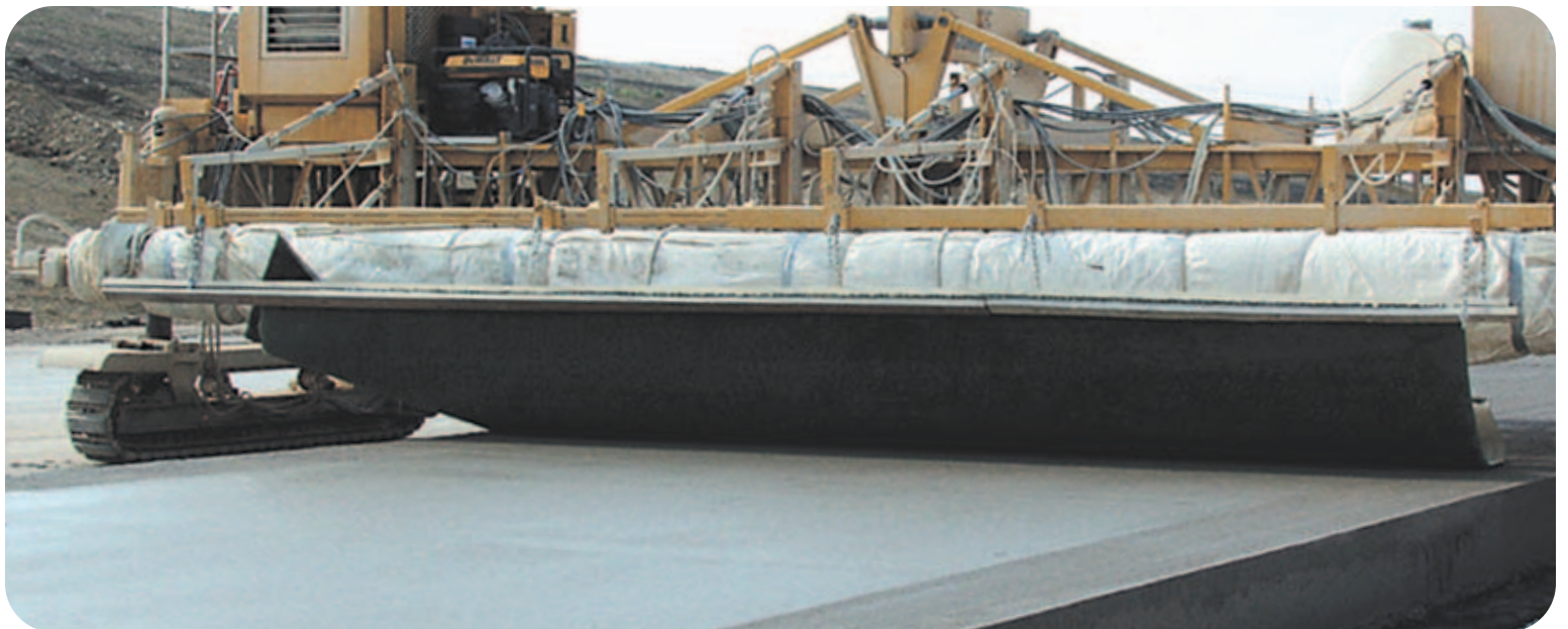
Versatility with the burlap/astroturf drag or poly-roll
