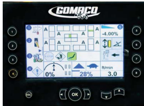
G+ Ground Control is available on the GP3. It's a remote operator's screen that can be positioned anywhere on the paver and allows the ground crew to see the same image that's on the operator's station. The crew can monitor their GSI readings, Trimble information and G+ operating status. Ground control also allows the ground crew to fine tune the paver and make adjustments to the settings.
