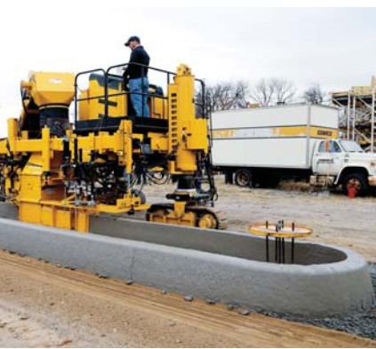
Turning a 24 inch (610 mm) radius -- The Commander III with rotary slew drives and extreme steering will turn a 24 inch (610 mm) radius or less. It's been proven in concrete at the GOMACO testing grounds in Ida Grove, Iowa.
