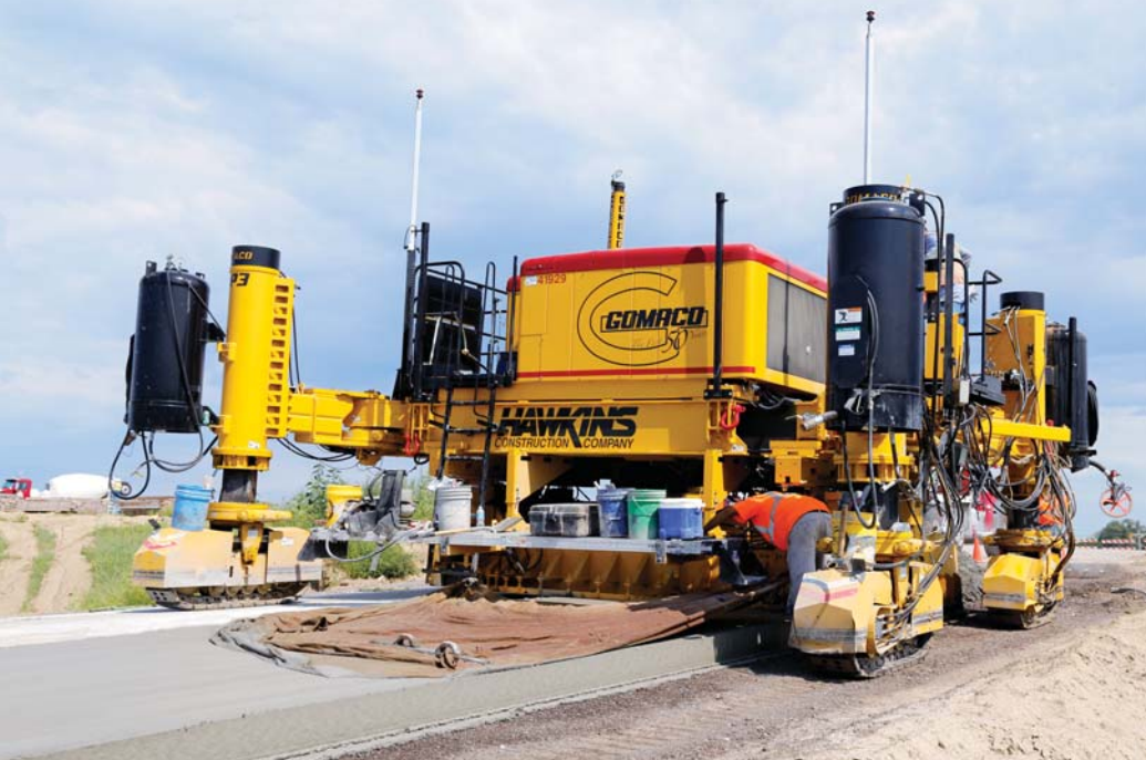
The GP3 is equipped with either a Leica Geosystems 3D guidance system or with a paver-mounted Trimble GPS system incorporating GOMACO sonic sensors.
