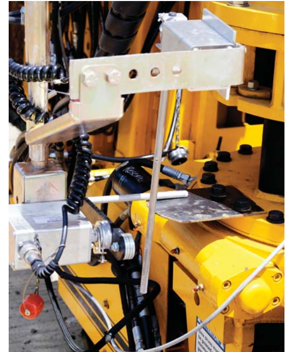
A steer wand sensing off a steel plate bolted to the back leg of the GP3 controls rear steering and grade. The GP3’s two right-side legs are locked to grade.
