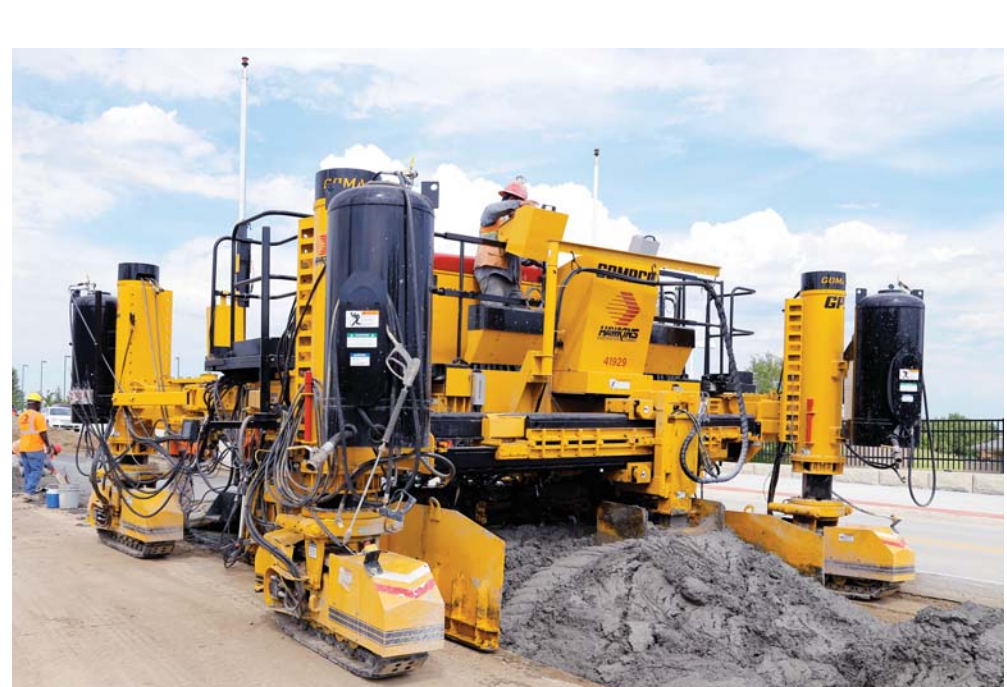
Hawkins Construction’s GP3 features a telescoping spreader plow on the front of the paver to move the concrete and to facilitate quicker width changes.
