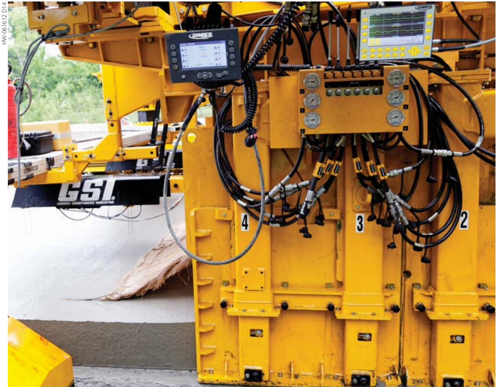
When scab-on paving, the GP3's steering wand on the front of the paver is sensing off the existing slab for grade and steering.
