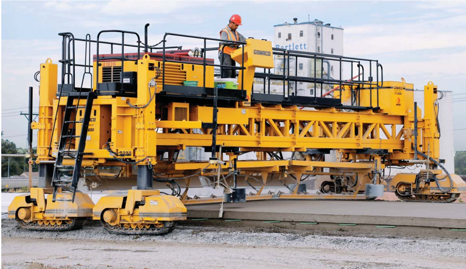
The new four-track T/C-5600 features patented technology along with GOMACO Tracer Texture Control to produce and maintain consistent tining depth.
