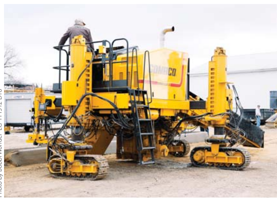
The rotary slew drives can turn the tracks at 90 degree angles to crab steer towards or away from stringline or other obstacles on a curb and gutter project.
