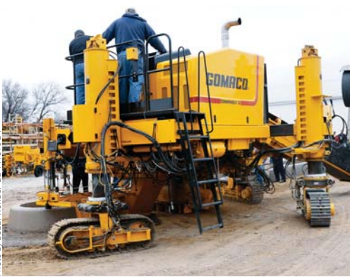
Turning a 24 inch (610 mm) radius -- The Commander III with rotary slew drives and extreme steering will turn a 24 inch (610 mm) radius or less. It's been proven in concrete at the GOMACO testing grounds in Ida Grove, Iowa.
