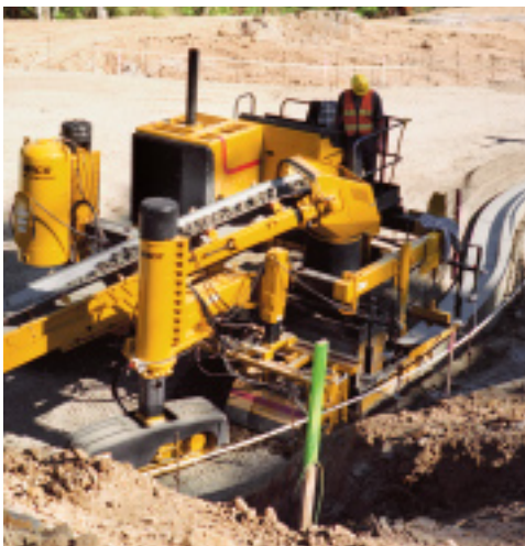
The Commander III trims and slipforms curb and gutter through a cul-de-sac. For clearance of obstacles, the three-track Commander III's trimmerhead and mold will hydraulically sideshift up to 36 in. (914 mm).
