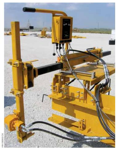
**1:** The operator moves the inserter apparatus to the forward or home position using the handle attached to the device.
