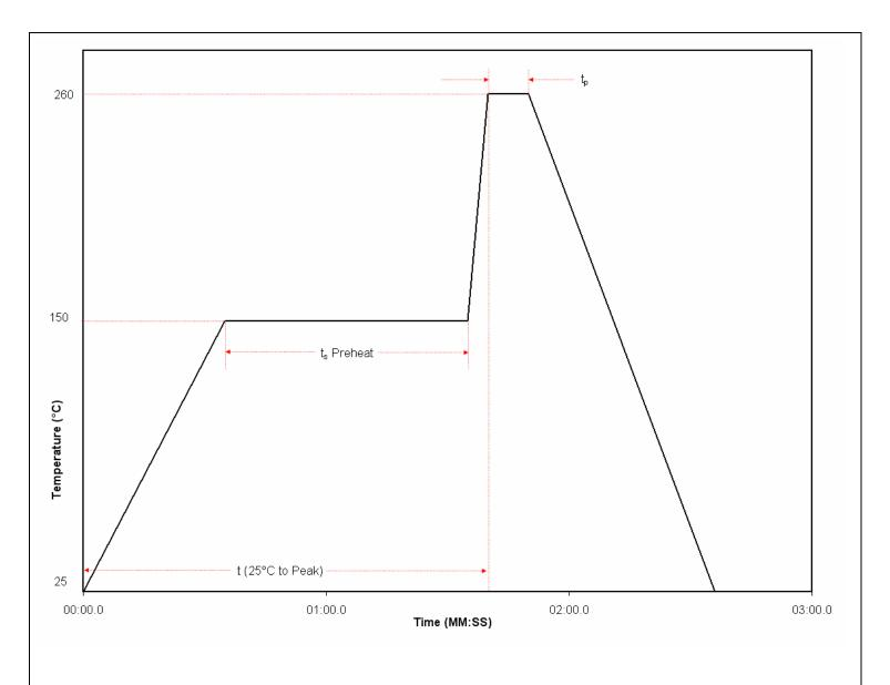
$t (25^{\circ}C \text{ to Peak}) = 100 \text{ seconds max}.$
