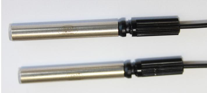
The LED Test Head has been designed to keep the intensity of the incident light stable when testing LEDs. The compact and robust design provides consistent and repeatable measurements.
