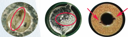
6R-S Razor witness marks on a lead-free pasted OSP VIA, no-clean process (left) and a lead-free pasted TEST PAD (middle) and an unfilled copper VIA (right)
