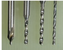
Drill A: Center Drill Drill B: Carbide Circuit Board Drill Drill C: Carbide Circuit Board Drill (with extended flute) Drill D: High Speed Steel Drill
