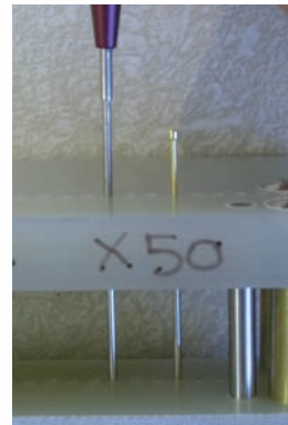
Proper use of termination extraction tool with spacer plate and probe plates installed.
