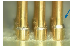
Figure C: The shoulder of the termination pin has been damaged due to excessive hammering of the tool. Inconsistent set heights may also occur.
