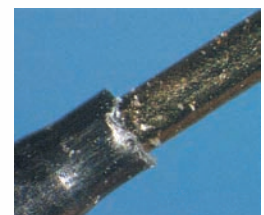
Damage to the socket tube will occur.
