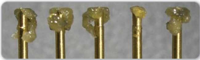
Actual photo of 8R Steel Razor still performing with a single actuation after 58,000 cycles on OSP, Lead-Free solder pasted (filled), No-Clean processed vias with heavy tip contamination.
