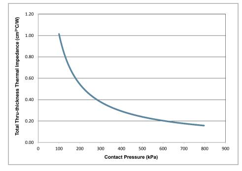
Thermal impedance reduces significantly with pressure
