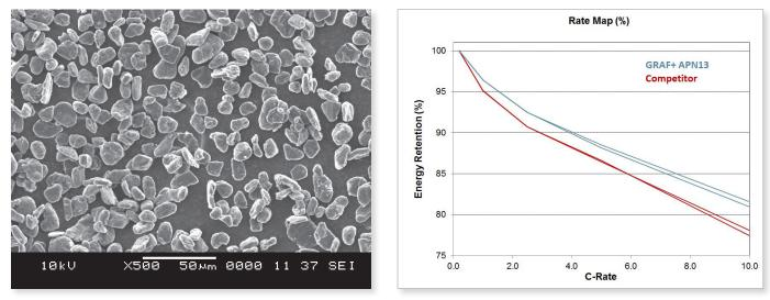
Outperforms competitive natural graphite anodes in retained capacity over a modified rate profile
