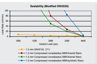
While maintaining an effective seal, GRAFOIL® material exhibits virtually no creep relaxation. As a result, the need for periodic bolt tightening is greatly reduced.
