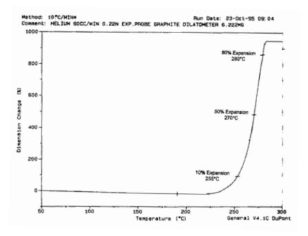
Figure 4: Thermomechanical Analysis (TMA) Plot for GP2 Intumescent Resin
