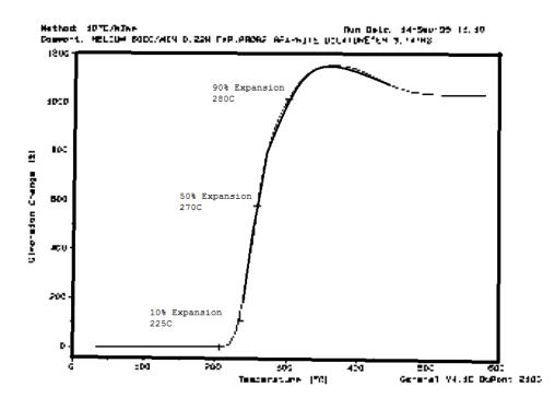
Figure 3: Thermomechanical Analysis (TMA) Plot for GRAFGUARD™ Grade 373
