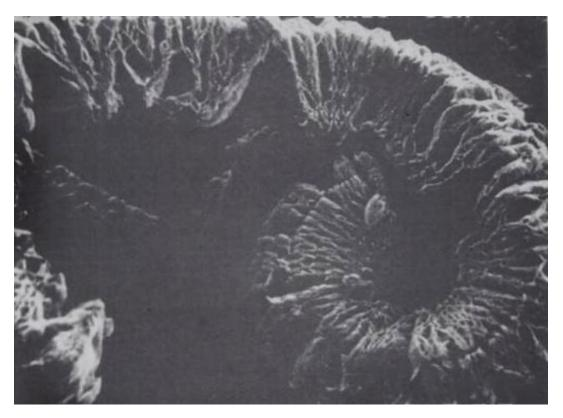
Figure 2: View of Expanded Graphite, magnified 50 times
