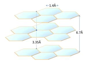
Figure 1: Crystal Structure of Natural Graphite Flake
