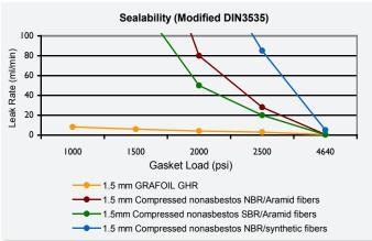
While maintaining an effective seal, GRAFOIL® material exhibits virtually no creep relaxation. As a result, the need for periodic bolt tightening is greatly reduced.
