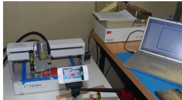
Figure 15: The T-Tech QuickCircuit 5000 PCB Prototyping System and host laptop running IsoPro 2.7.
