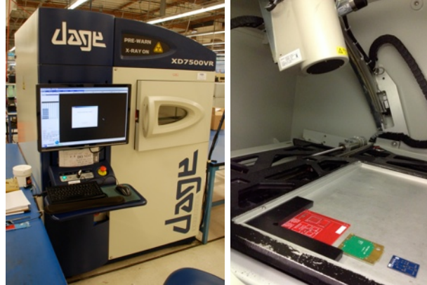
Figure 20: The DAGE XD7500VR X-ray System (left) and inside the X-ray chamber (right).
