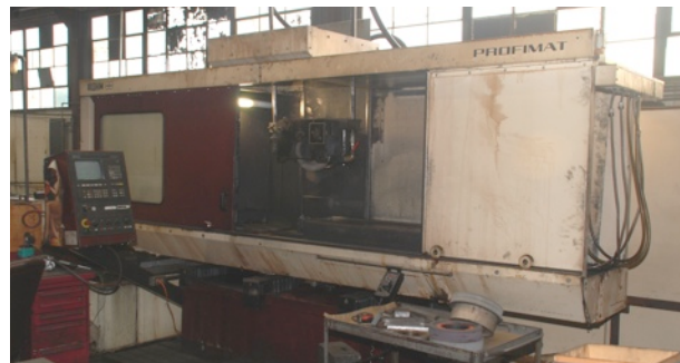
Figure 18: The Blohm PROFIMAT CNC Creep Feed Surface Grinder with a Siemens SINUMERIK 810G controller.
