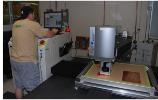
Figure 11: The LPKF MicroLine 600D UV Laser System.
