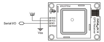
The on-board, four-pin, 0.1"-pitch header allows the GPS Receiver Module to easily be plugged into a solderless breadboard or prototyping PCB. If the default "Smart Mode" is desired and the /RAW pin will be unused, the Module can be simply connected to its host with a standard three-wire servo extension cable (for example, Parallax #805-00001).
