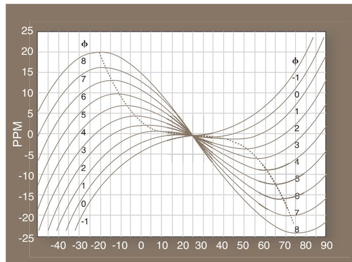
Figure 1. Family of characteristic temperature curves for fundamental frequency of AT-cut crystal.
