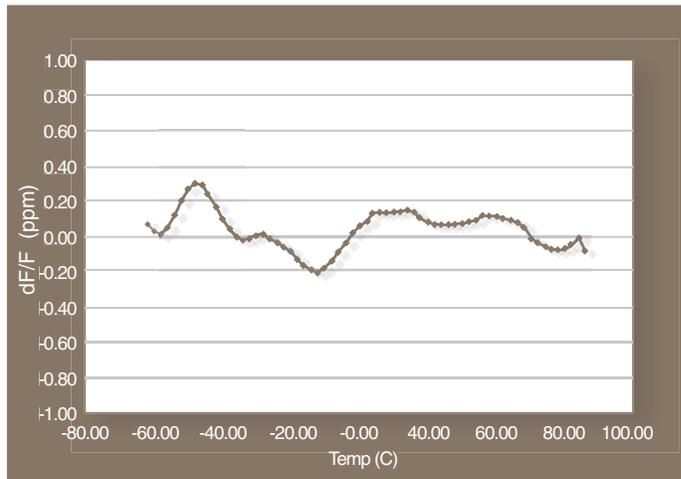
Figure 3. Frequency vs. temperature of 20MHz TCXO at 2°C intervals.
