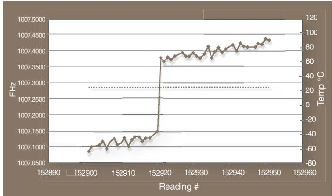
Figure 6. Expanded view of 10 ppb micro-jump.
