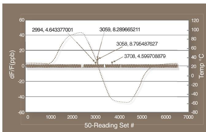
Figure 5. First difference between successive continuous frequency samples.
