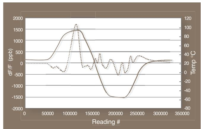
Figure 4. 20MHz TCXO frequency during a °C/minute temperature ramp.
