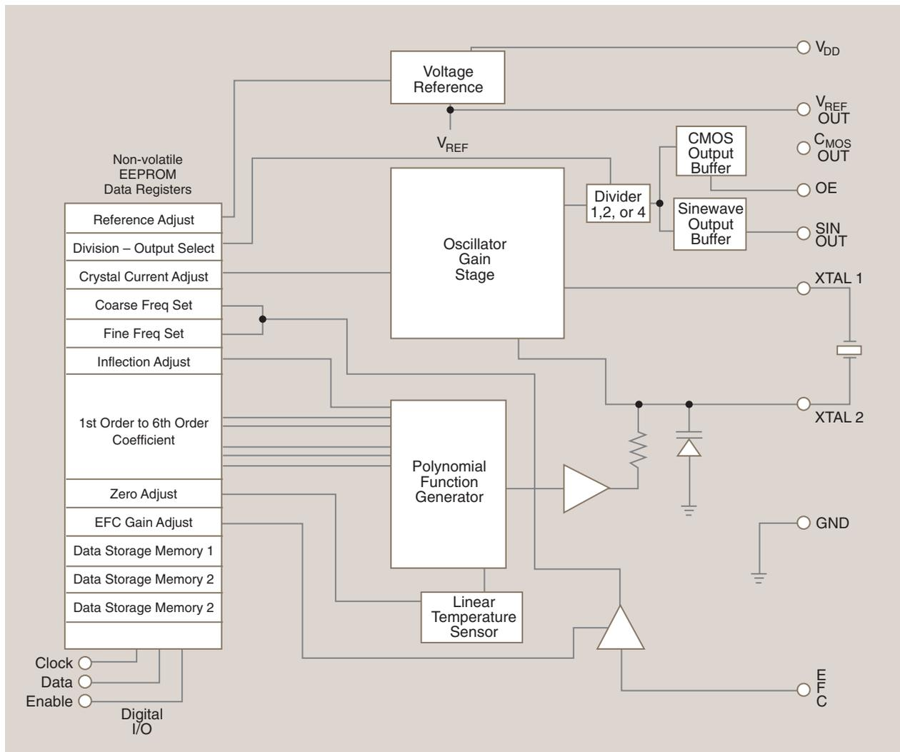
Figure 2. Integrated TCXO ASIC.
