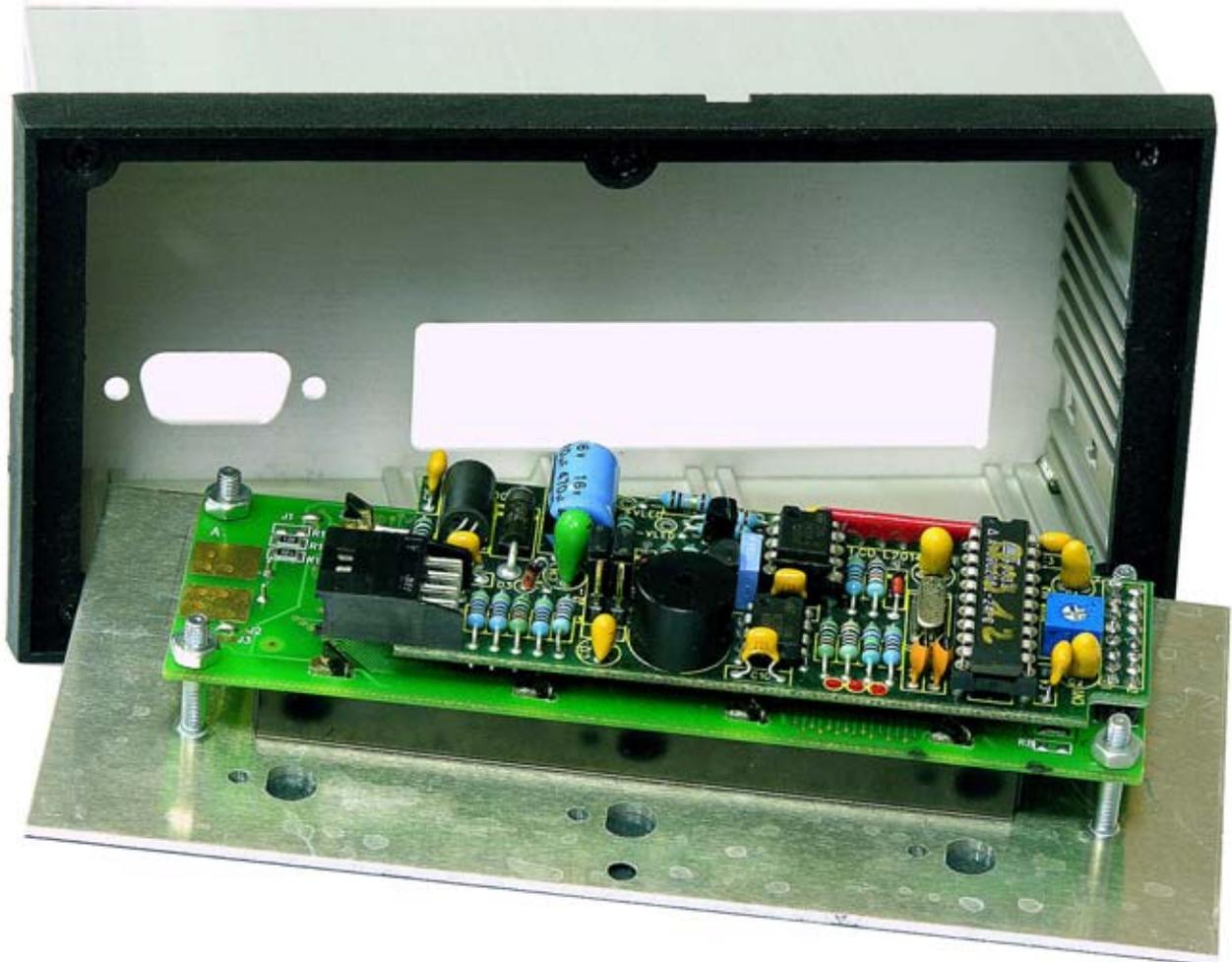
**FIGURA C1: MONTAGGIO TRAMITE CONTENITORE METALLICO**
