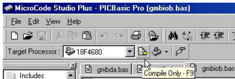
FIGURE 30: COMPILING THE PROGRAM WITH MICROCODE STUDIO + PIC BASIC PRO
