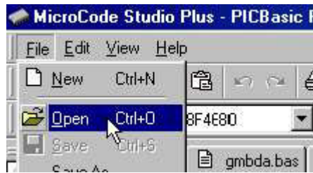
FIGURE 29: LOADING SOURCE FILE WITH MICROCODE STUDIO + PIC BASIC PRO
