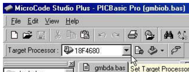
FIGURE 28: SELECTING TARGET PROCESSOR WITH MICROCODE STUDIO + PIC BASIC PRO
