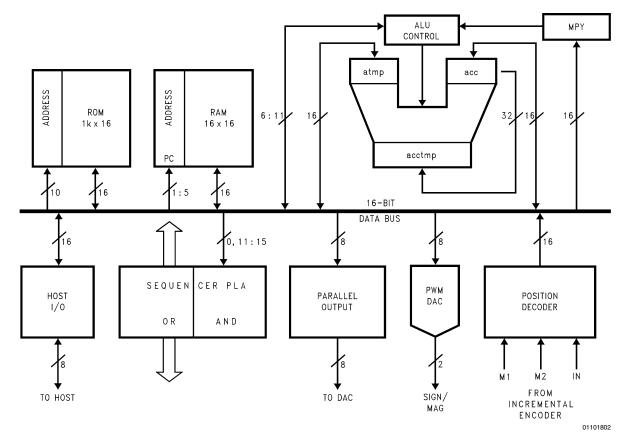
FIGURE 2. Hardware Architecture of LM628/629
