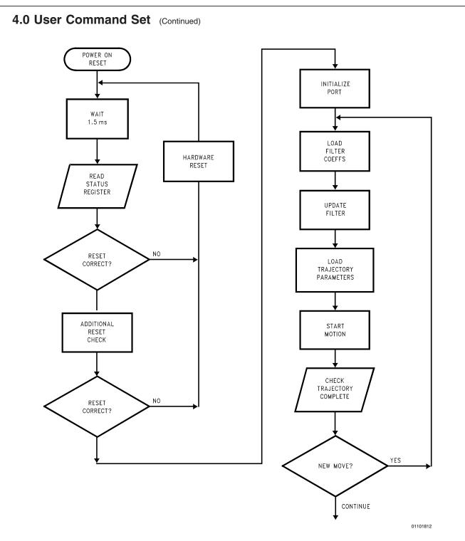
FIGURE 12. Basic Software Flow
