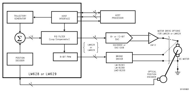
FIGURE 1. LM628 and LM629 Typical System Block Diagram
