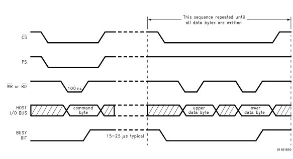
FIGURE 10. Busy Bit Operation during Command and Data Write Sequence
