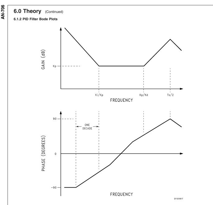
FIGURE 17. Bode Plots of PID Transfer Function
