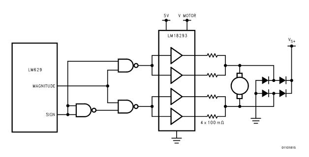
FIGURE 15. LM629 H-Bridge Motor Drive Example Using LM18293
