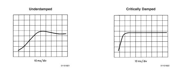
FIGURE 11. Position vs Time for 100 Count Step Input
