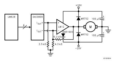
FIGURE 14. LM628 Example of Linear Motor Drive Using LM12
