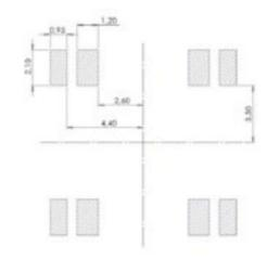
All dimensions in mm Tolerances unless otherwise specified: ±0.20mm Pins coplanarity 0.15mm
