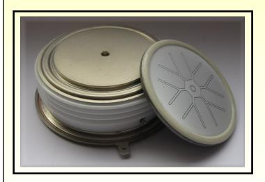
pressure contact distributed gate thyristor with increased power density. This new fast thyristor with turn-off time of as little as 20µs and current rating 1955A, is symmetrical blocking with Vdrm/Vrrm equal to 1600V and therefore suitable for both voltage and current fed applications.
