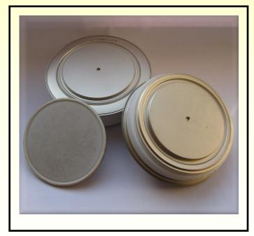
IXYS UK Westcode Ltd. Adds three new voltage classes to its range of 83mm die, pressure contact rectifier diodes; the new introductions are at 1.5kV, 4.0kV and 4.8kV. These devices use bonded die technology and improved package design, to give a significant improvement in power density over older designs within the same package footprint, as well as better electromechanical & thermal performance.
