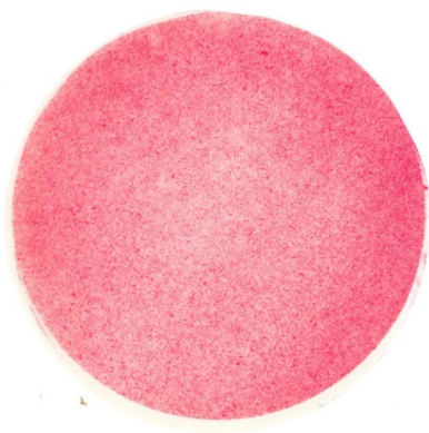
Example of good pressure distribution
