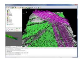
Use LiDAR point cloud data to identify trees and power lines that need to be kept clear of encroaching vegetation.
