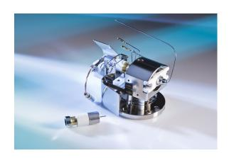
The Model 7535MH5 and 7596MH5 are Harris channel electron multiplier (CEM) assembly used in Agilent 5973 MSD mass spectrometers. The monolithic ceramic construction and advanced ion-optical design significantly extend multiplier life, enhance sensitivity, and offer greater linear dynamic range. Its exclusive snap-out/snap-in mounting both speeds multiplier replacement and assures perfect alignment.
