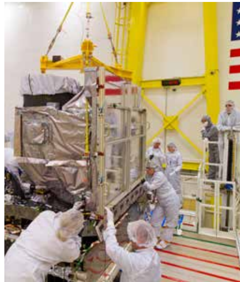
Installation of ABI on GOES-R
