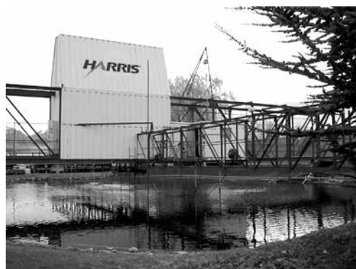
Harris largest in-water acoustic test facility is 60 feet long and 35 feet deep.
