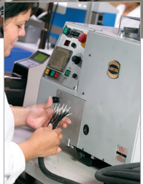
Programmable insulation strip/crimp machine handles many types of cable
