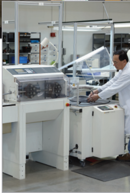
Automation machinery measures cuts to length, de-jackets, and coils cable at a specific station
