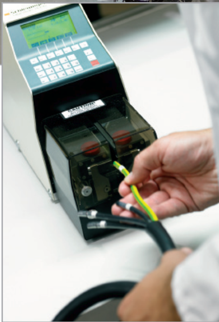
Programmable insulation stripping machine handles many types of wire
