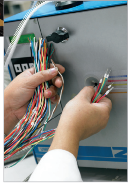
Automated strip and crimp ferrule installation
