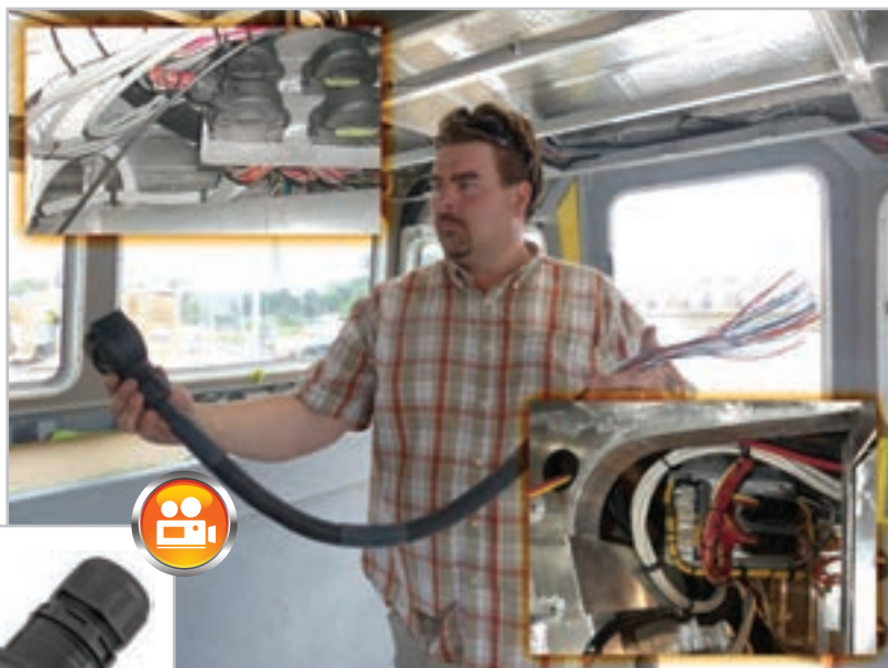
MetalCraft Marine assistant supervisor Shawn Latreille holding a wire assembly with a Han-Eco termination. Top left above: Mated wire bundles with Han-Eco. Bottom right above: Han-Eco installed in hull. Left: With the help of Harting Han-Modular inserts, Han-Eco heavy-duty connectors can carry a combination of power, signal, fibre optic, coax, D-Sub and pneumatic through the same unit. (Cover photo courtesy MetalCraft Marine.)
