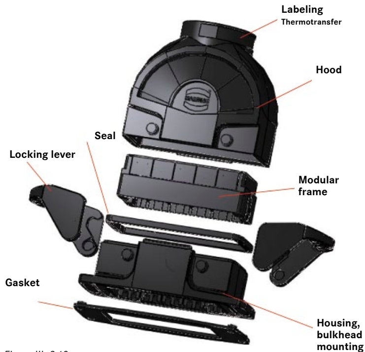
Figure III- 2.10 Overview of the Han-Eco® hood and housing
