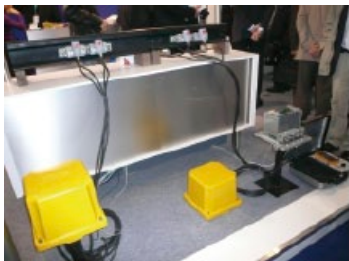
Figure II- 8.1 The axle counter system
