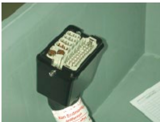
Figure II- 13.4 Han-Modular® contact inserts with Quintax, EE module and Han® 46 EE: mounted in the Han® M hood, size 48 B.
