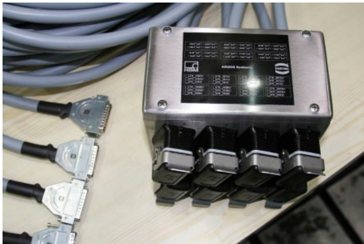
Figure VI- 5.1 Stainless-steel distributor box, Heavy Duty Connectors and pre-assembled D-Sub cables
