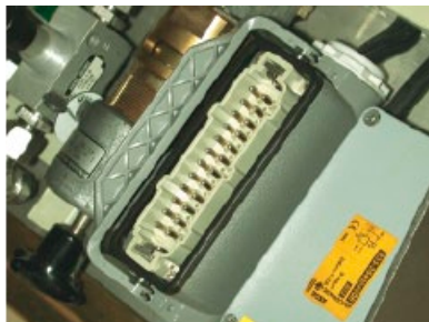
Figure II- 12.2 Detailed view of the Han® 24E connector that is built into the controlling device for the DSA 200 pantograph
