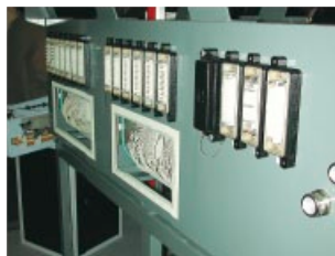
Figure II- 10.3 Sub-floor container, back side with the HARTING Han® connectors
