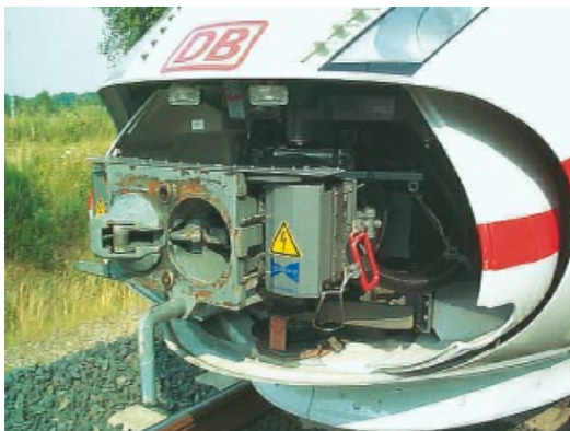
Figure II- 13.1 Opened front hatch on an ICE3 train The coupling unit is easy to see. The contacts for the electrical connections between the coupling units are covered. The control unit (refer to Figure II- 13.2) for the front hatch (not visible here) is located directly behind the coupling unit.
