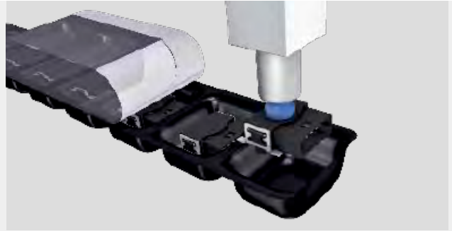
Reflow and SMD-solderable components for automated mount and soldering processes
