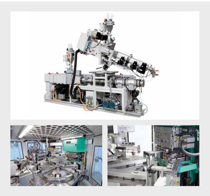
Courtesy of: KraussMaffei Technologies GmbH (Fig. 1: co-extrusion facility for window profile production) ARBURG GmbH & Co. KG and ZAHORANSKY AG Systemtechnik (Fig. 2, 3: production cell for medical devices)
