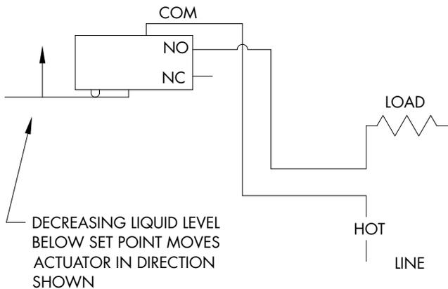
**Fig 2:** Wiring schematic for power applied to load when liquid level is greater than set point (power to load interrupted when level decreases to below set point).
