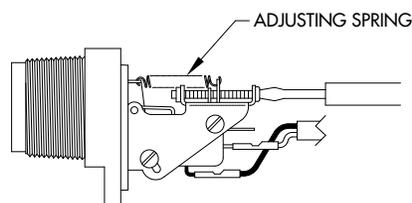
3. Insert blade type screw driver in the slotted end of the adjusting screw and turn it in a clockwise direction. This extends the length of the adjusting spring, which in turn adjusts the float net effective buoyancy to respond to lower specific gravity fluids.
