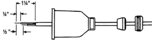
3. Remove slip-on connectors from microswitch and crimp or solder to the leads.
