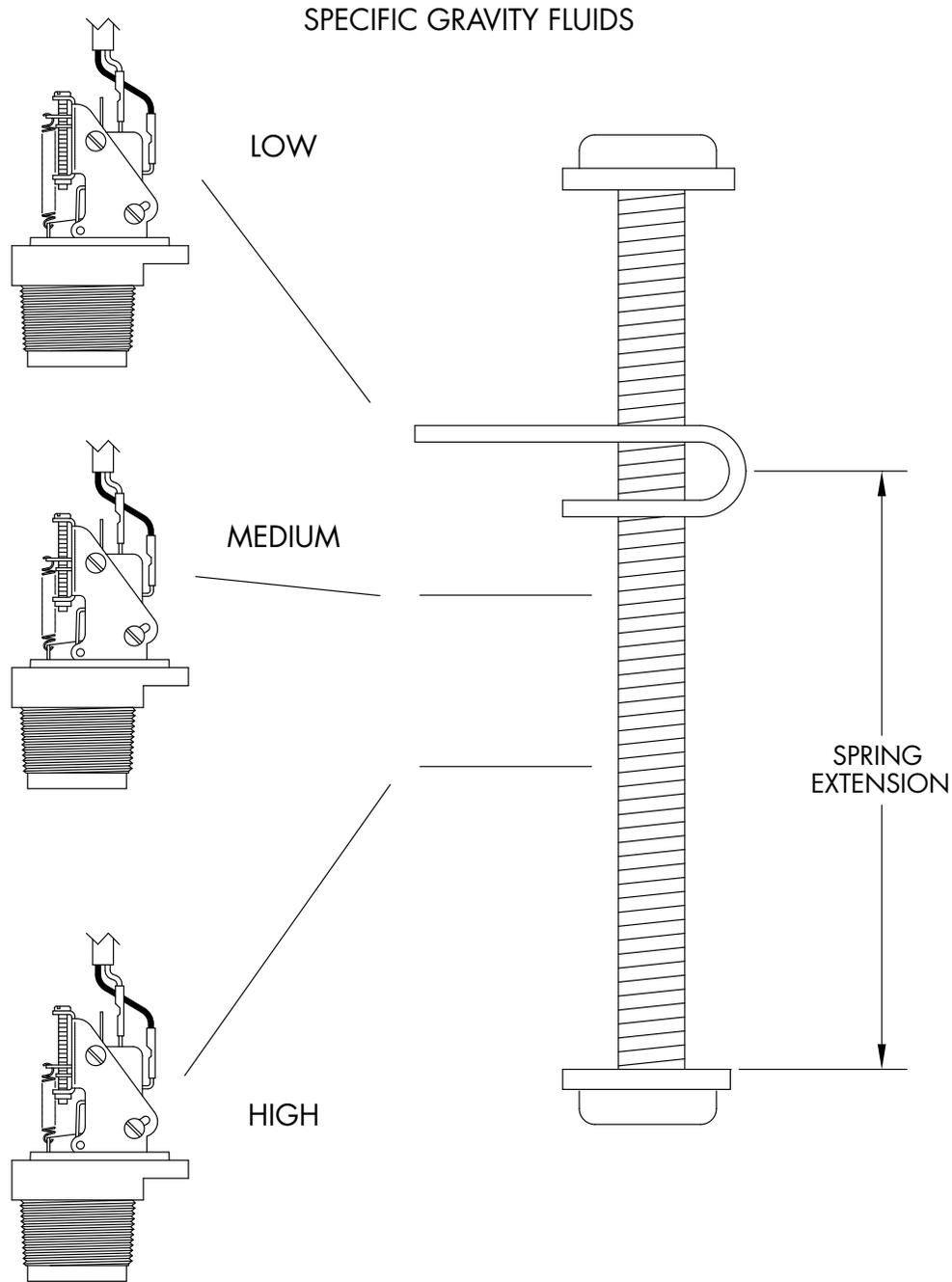
Microswitch actuation point may be monitored during the adjustment procedure detailed in (2 and 3) above by an audible click or with an ohmmeter before connecting line power to the terminal strip, or by monitoring the voltage supplied to the load through the microswitch.
